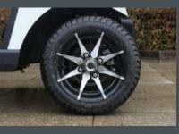
12 inch aluminium rim wheel with low profile tire 215/35-12 (Optional for 2-4 seats, standard for 4 seats with cargo box and 6 seats)
