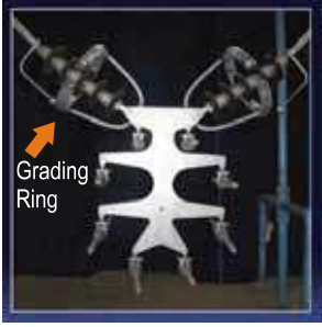
1200kV Single V Suspension String for Octagonal Bundle with CC Rings
