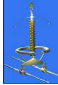
400kV Single Suspension Twin Bundle Assembly
